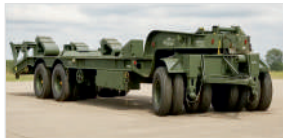
50 Ton Mechanical Trailer: Heavy Duty Tank Transporter
