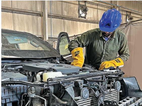
Stock or factory production vehicles undergo structural engineering with special grade ballistic steel reinforcements, besides other functional areas like windows, tyre and wheels.
